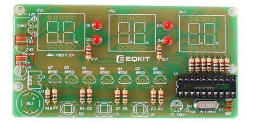
Step 9:Install 1pcs XH2.54mm-2P Socket Right Angle Socket at J2.
